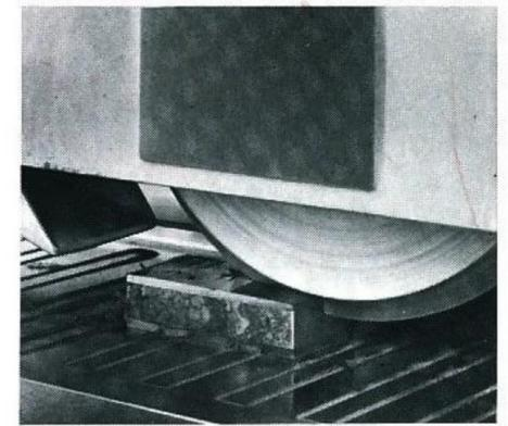
Creep feed grinding from the solid: it always has been standard feature of the MHPE 500
